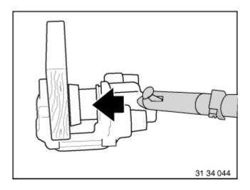
Press out piston with compressed air applied through connection bore.
