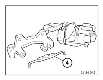
Dismantle brake caliper and remove brake linings. **Installation**:
