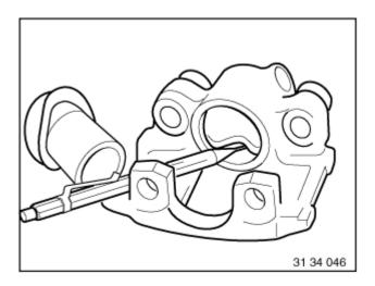
Remove sealing ring carefully with a plastic needle.
